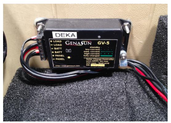
A Genasun GV-5 charge controller is attached to the inside of the Pelican case and is pre-wired to connect to the solar panel, batteries and power the GPS receiver.
