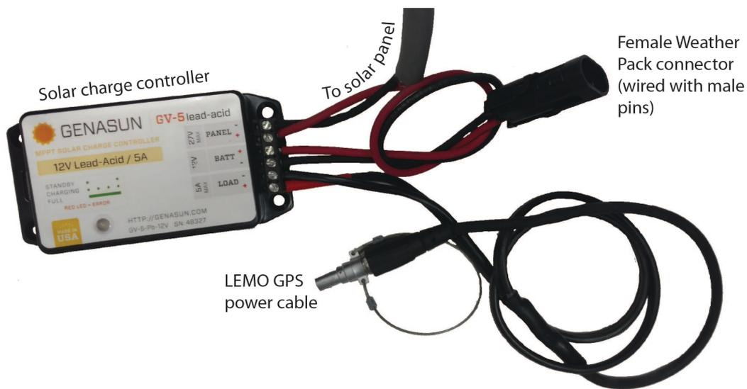
A Genasun GV-5 charge controller is attached to the side of the Pelican case with Velcro and is pre-wired to connect to the solar panel, batteries and power the GPS receiver.
