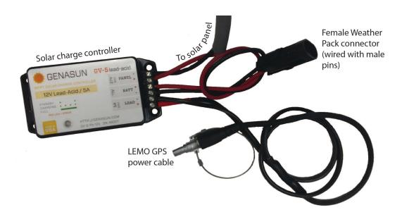
A Genasun GV-5 charge controller is attached to the side of the Pelican case with Velcro and is prewired to connect to the solar panel, batteries and power the GPS receiver.
