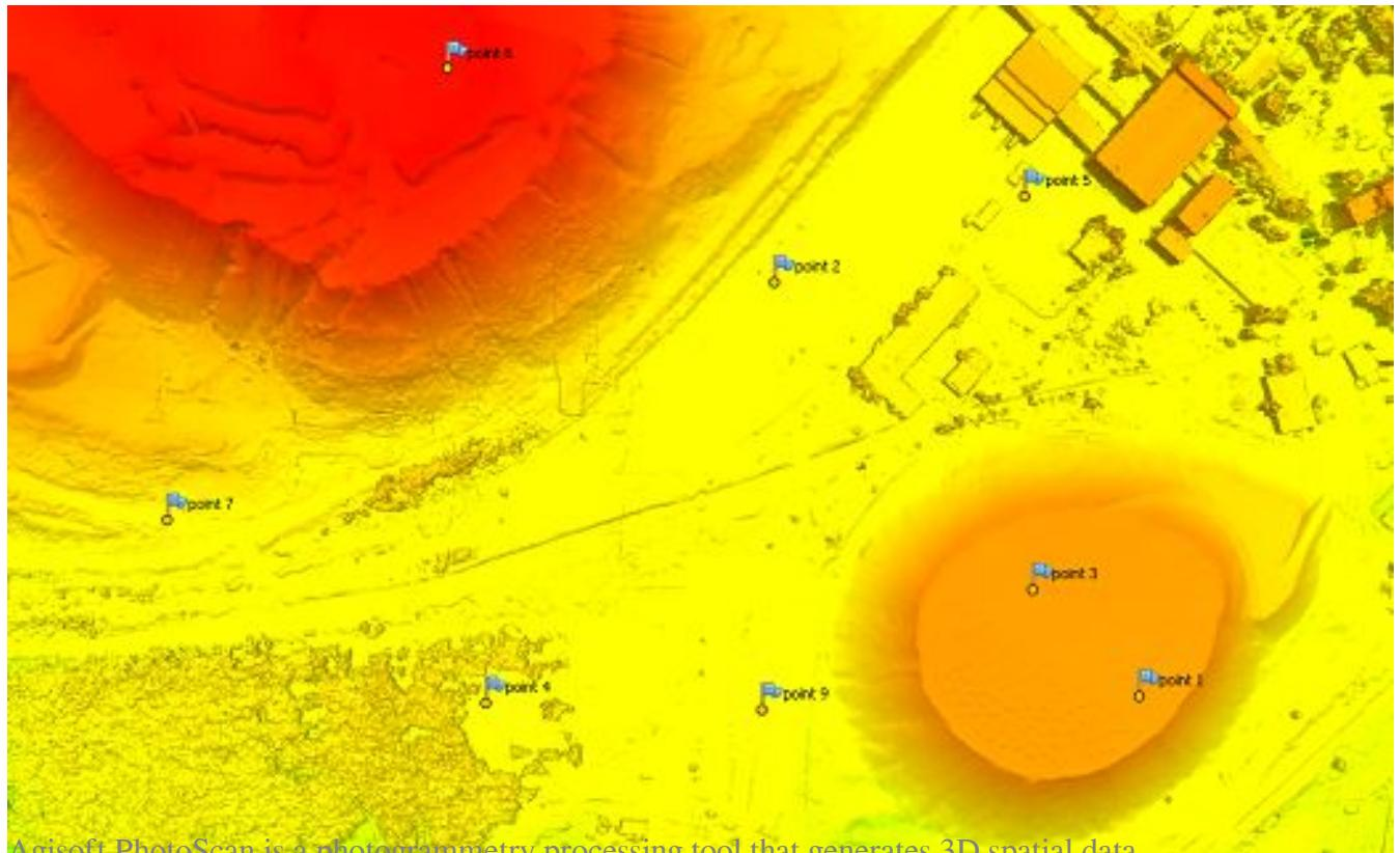
Agisoft PhotoScan is a photogrammetry processing tool that generates 3D spatial data.
