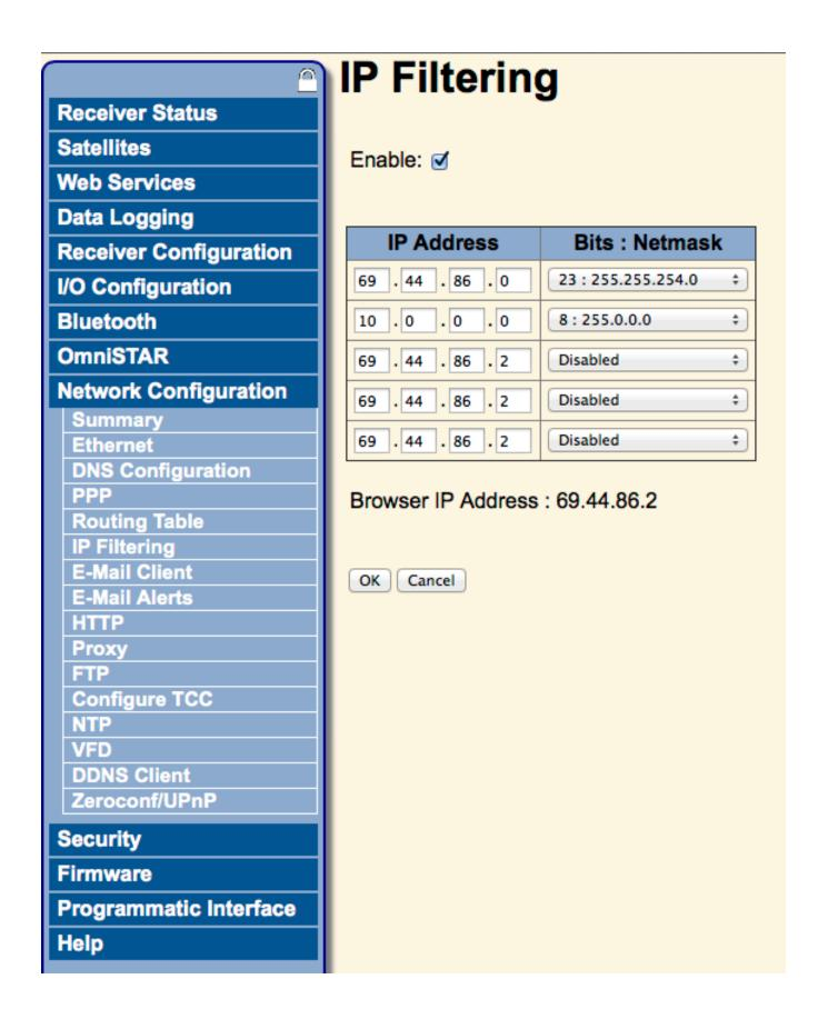
Enter all of the IP addresses that will need access to the receiver. Specify the required <u>Netmask</u> for each address. Then select 'OK' to save the changes.
