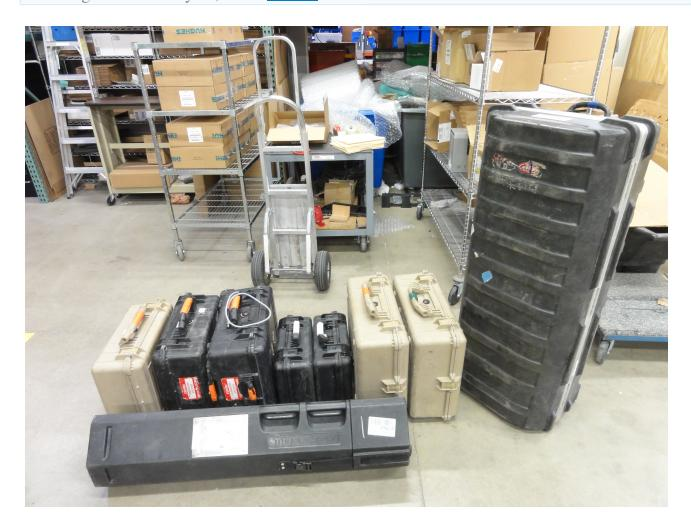
The basic kits for each of our Riegl Terrestrial Laser Scanners (TLS) are comprised of 5 to 7 Pelican cases, 1 tripod case, and 1 SKB 1SKB-H5020W railpack utility case per scanner. The image above is an example of what a typical TLS kit looks like.
