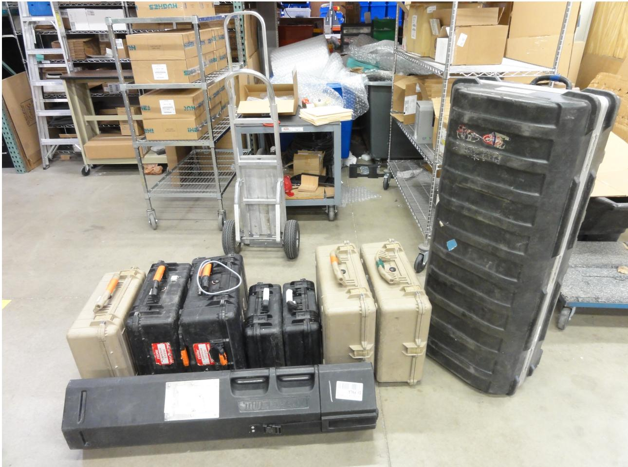
The basic kits for each of our Riegl Terrestrial Laser Scanners (TLS) are comprised of 5 to 7 Pelican cases, 1 tripod case, and 1 SKB 1SKB-H5020W railpack utility case per scanner. The image above is an example of what a typical TLS kit looks like.
