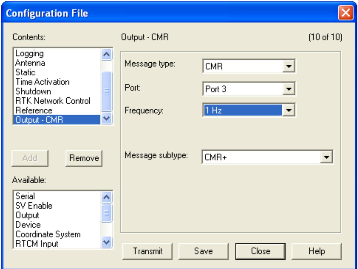
6. Select the 'Coordinate System' tab from the 'Configuration File' window. If it is in the bottom list, under 'Available,' select it and hit the 'Add' button.
