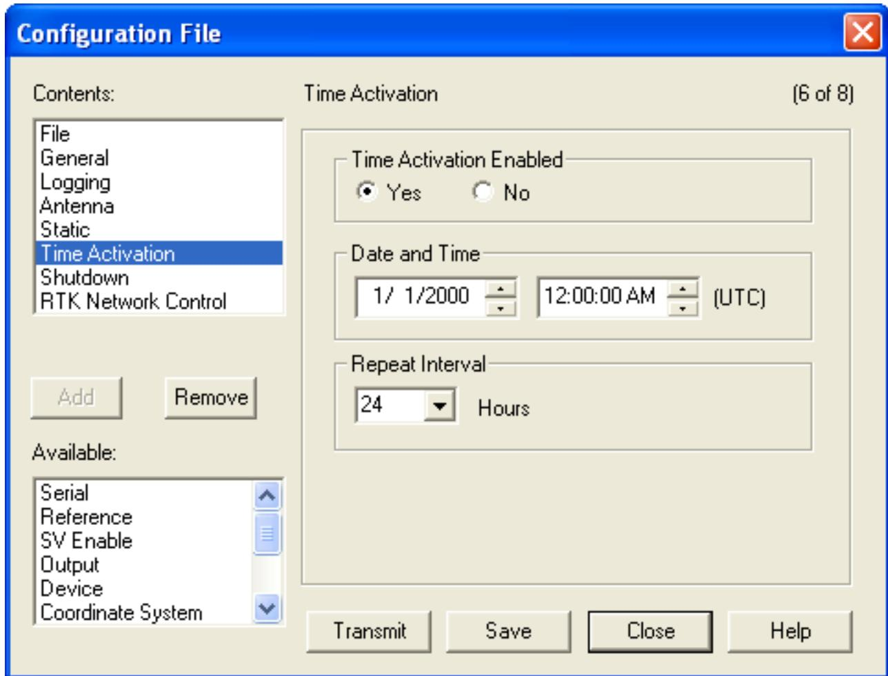
'Time activation' and the subsequent options direct the receiver when to start and stop data logging. The options shown result in daily (24 hour) data files starting at 0:00 UTC. In this case, the 'Date and Time' are not important, so long as the specified start time is before the current survey.
