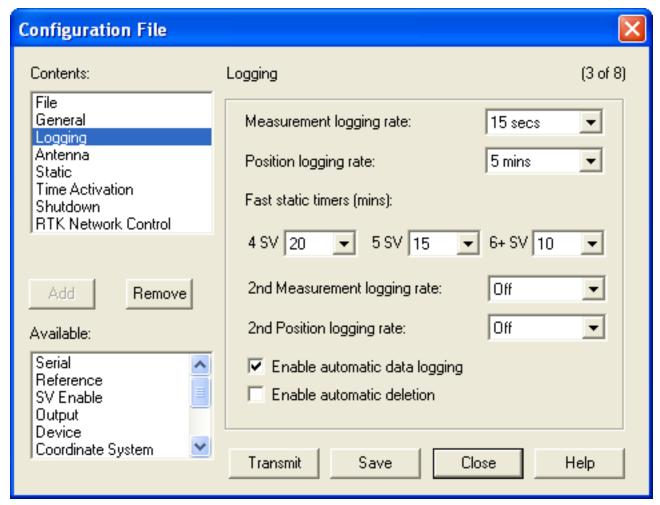
You may want to change the 'Measurement logging rate.' 'Enable automatic data logging' directs the receiver to automatically start logging data upon power up. This is important is situations where the receiver may lose and regain power.
