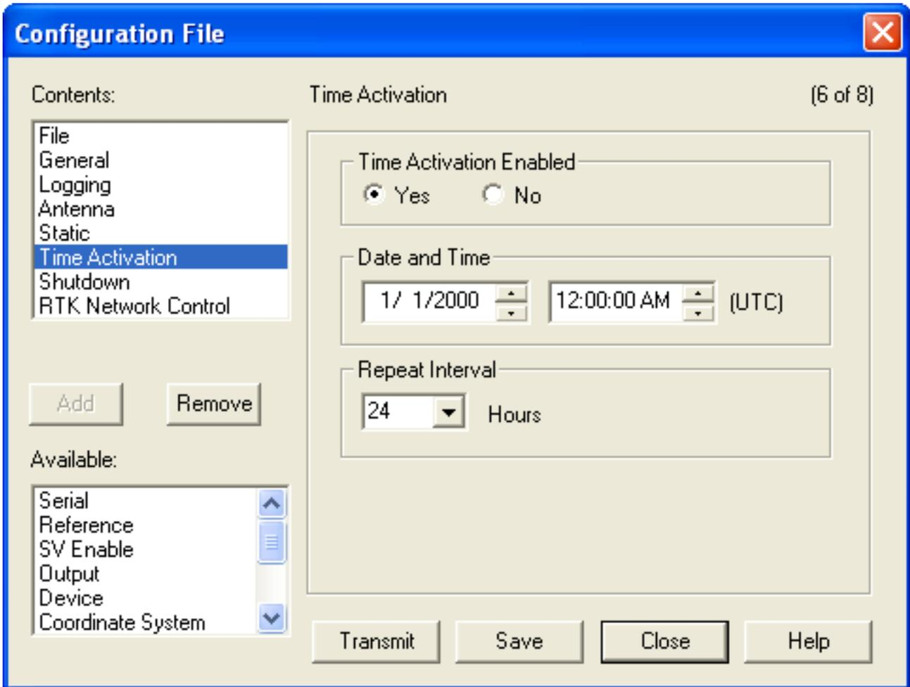
'Time activation' and the subsequent options direct the receiver when to start and stop data logging. The options shown result in daily (24 hour) data files starting at 0:00 UTC. In this case, the 'Date and Time' are not important, so long as the specified start time is before the current survey.
