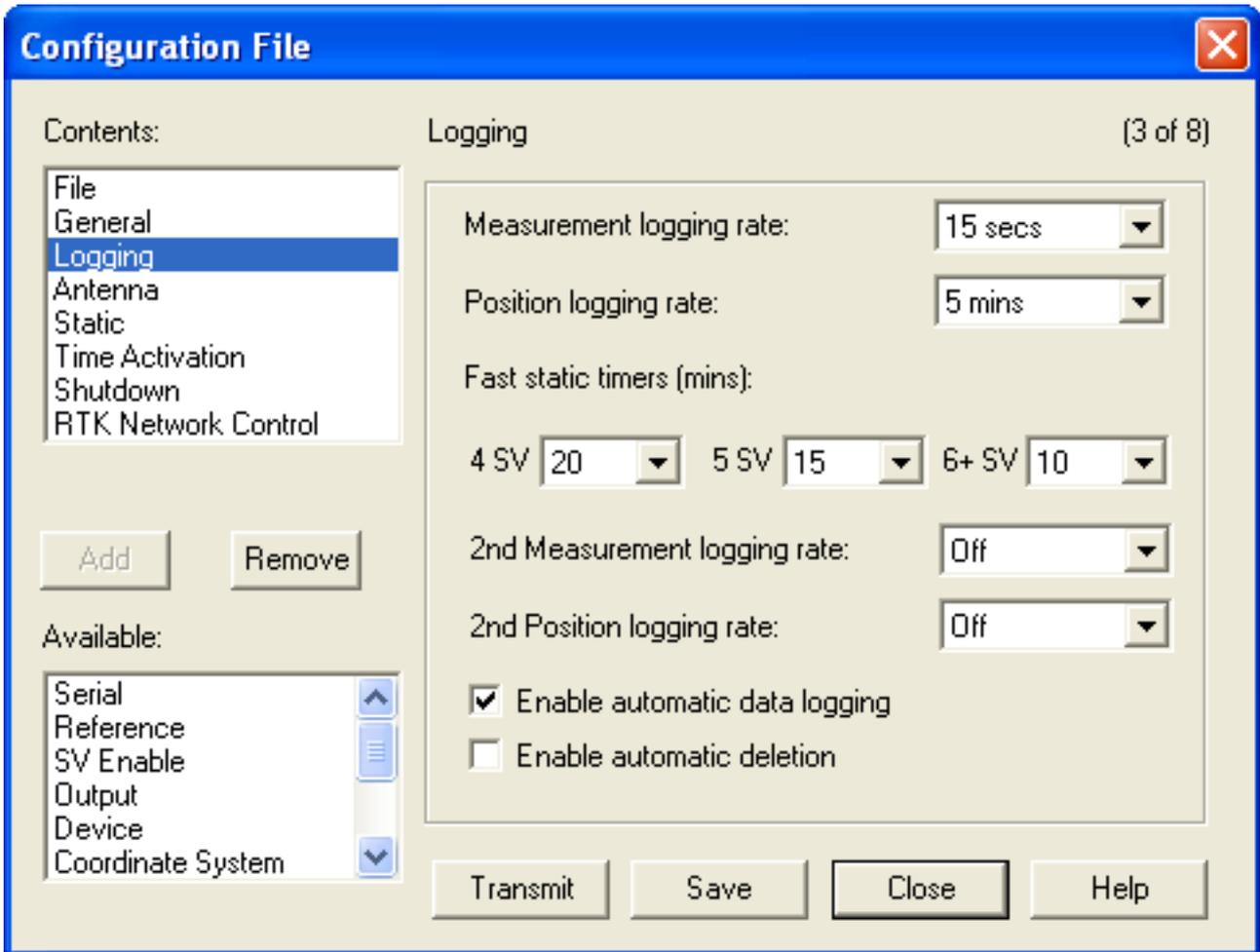
You may want to change the 'Measurement logging rate.' 'Enable automatic data logging' directs the receiver to automatically start logging data upon power up. This is important in situations where the receiver may lose and regain power.
