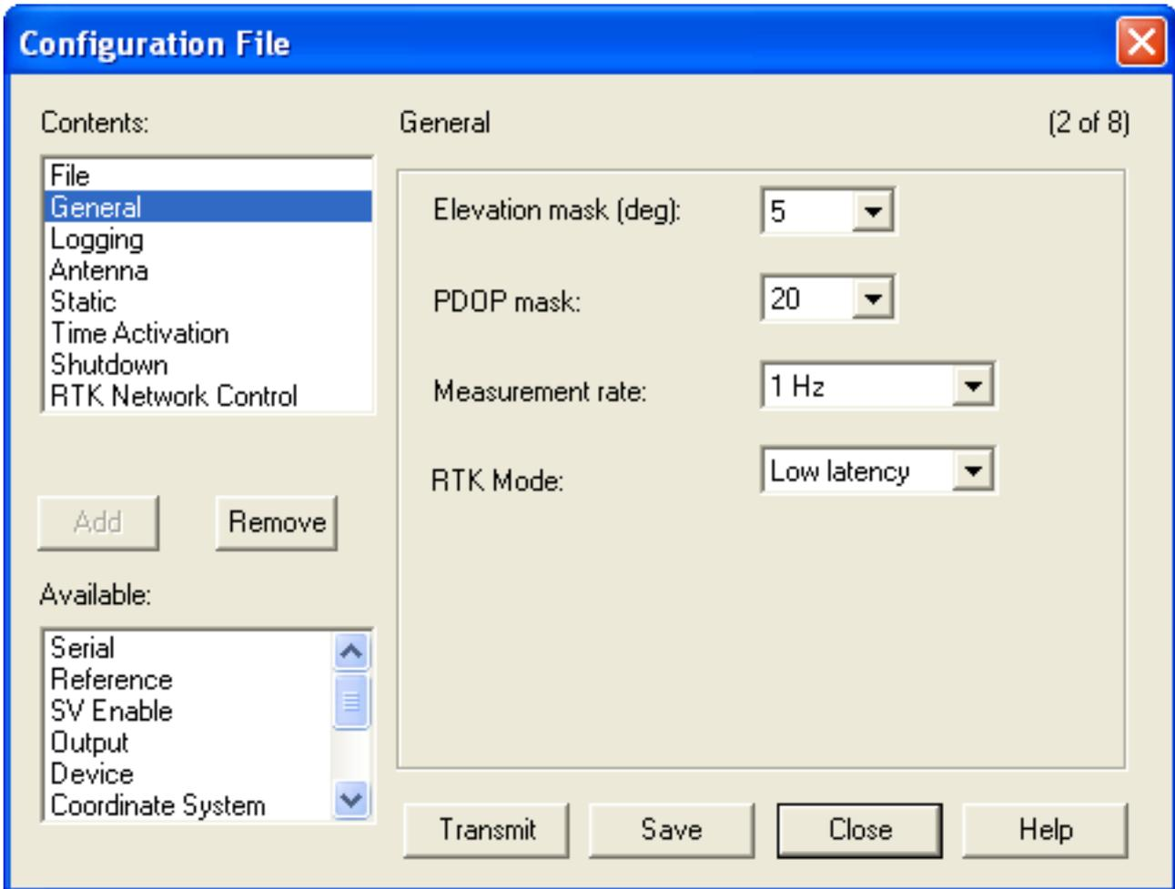
Elevation mask is the angle above the horizon below which no satellite data are collected.
