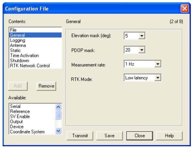
Elevation mask is the angle above the horizon below which no satellite data are collected.
