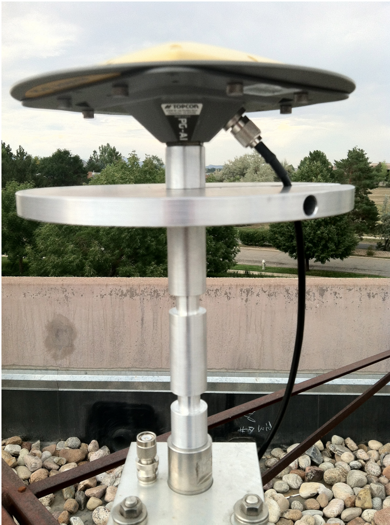
Figure 2. The antenna testing mount with TPSPG_A1+GP type antenna in place (looking north). The testing mount consists of an aluminum standoff with three evenly spaced notches that allow for a aluminum disk to be precisely fixed at different heights below the antenna. The disk can be moved without displacing the antenna.
