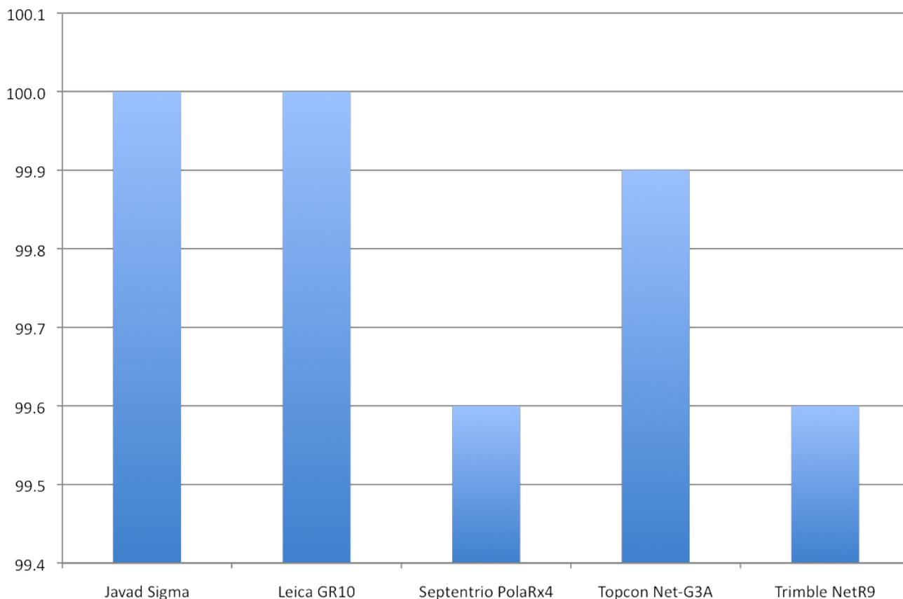
The following figures show the average number of detected cycle slips that occurred during our 5-day test. The upper figure shows the number of slips that were detected for satellites with elevations angles greater than 10 degrees. The lower figure shows the number of slips that were detected for satellites with elevation angles less than 10 degrees.
