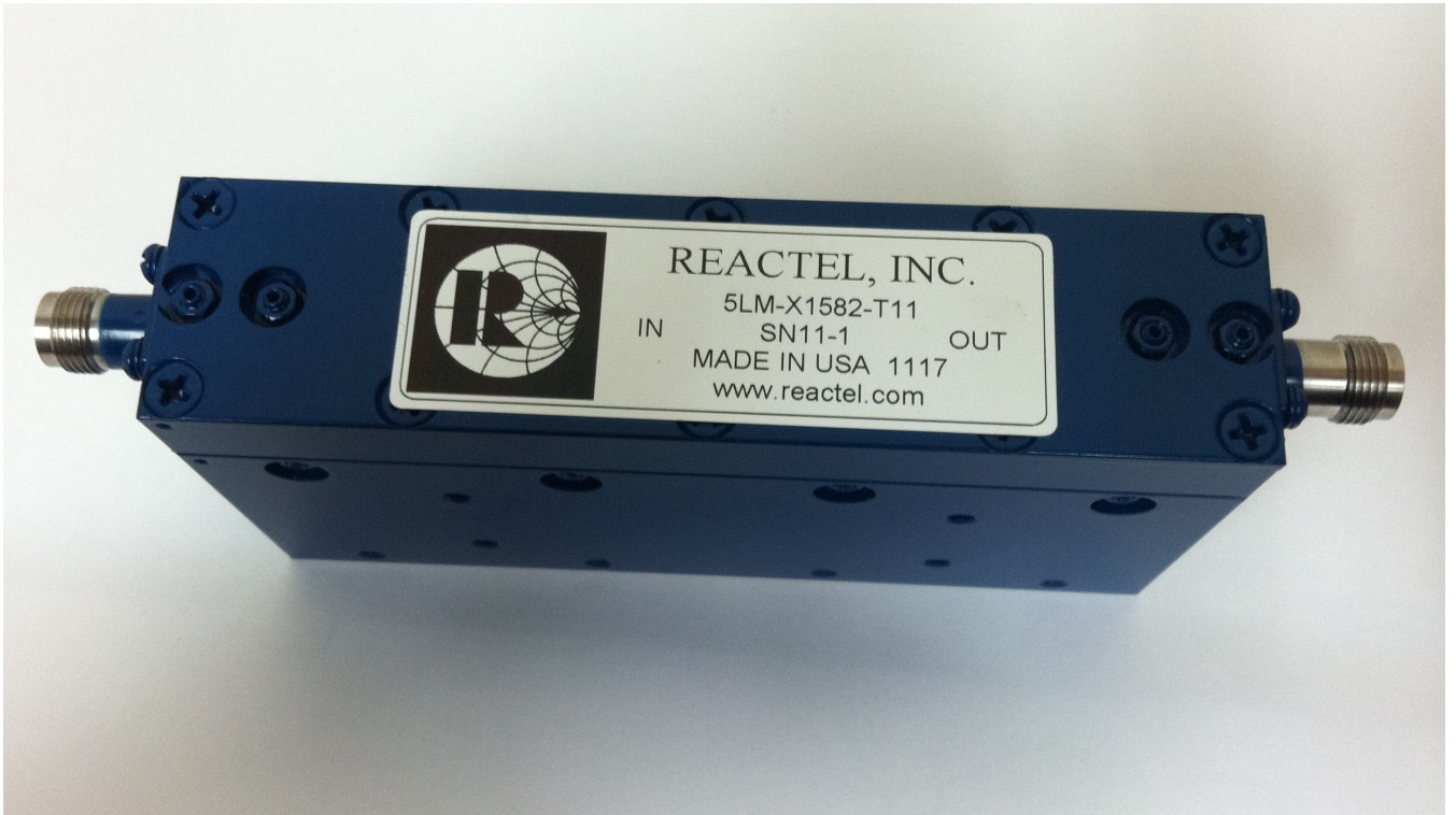
Above: A custom cavity-type notch filter designed to mitigate the interference caused by Iridium communication transmissions.
