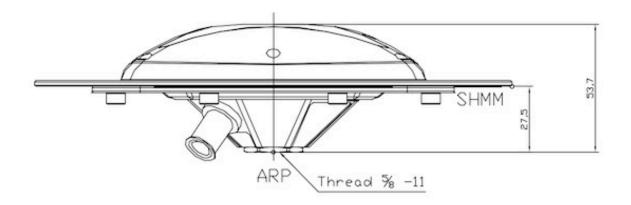
Dimensions are in mm ARP - Antenna Reference Point SHMM - Slant Height Measure Mark
