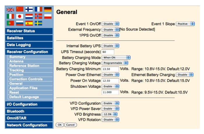
2. If a Charge Controller WITH an LVD is used: identify the voltage thresholds of the LVD and set the receivers voltages below each of them. A commonly used controller - the <u>Flexcharge NC30</u> - will disconnect the load when battery voltage drops below 10.9V and reconnect at 12.9V. The NetR9 should then be set to:
