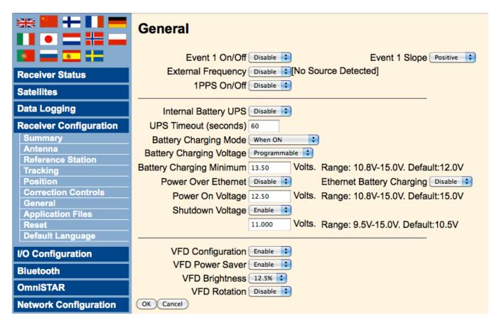
2. If a Charge Controller WITH an LVD is used: identify the voltage thresholds of the LVD and set the receivers voltages below each of them. A commonly used controller - the <u>Flexcharge NC30</u> - will disconnect the load when battery voltage drops below 10.9V and reconnect at 12.9V. The NetR9 should then be set to:
