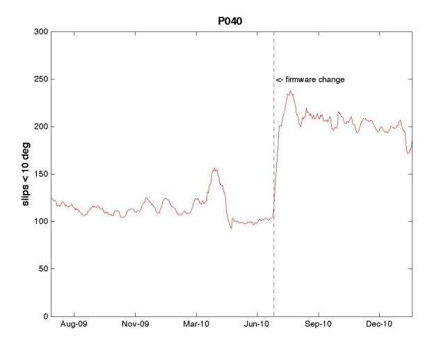
The following figure shows 24-hour totals of MP or IOD slips that occur at the site P040 when the
