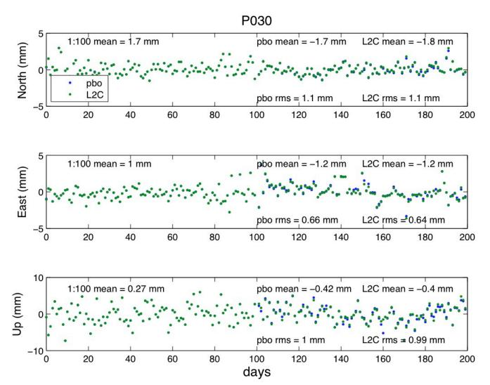
The mean differences between the position time series are  $< \sim 0.1$  mm in the horizontal and  $< \sim 0.2$  mm in the vertical components (shown below).
