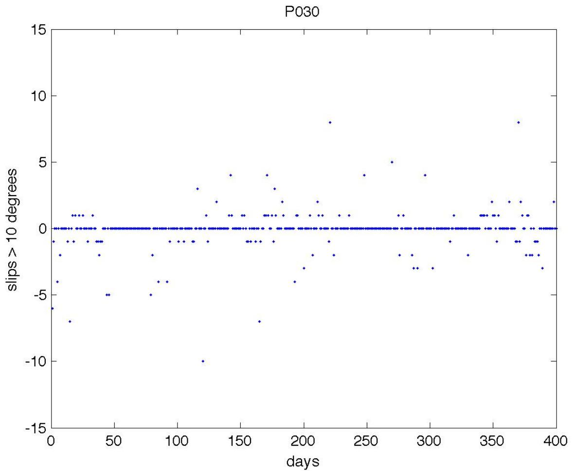
We have observed that for elevation angles  $< 10^\circ$  the mean difference between the number of slips for L2C and L2P phases is  $\sim 7.7$  slips over a 400 day period. Tracking L2C increases the number of observations, but it also increases the number of slips for elevation angles  $< 10^\circ$ .
