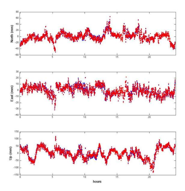
The following figure shows the difference between the L2P and L2C analyses when using one receiver that corrects for the 1/4-cycle bias and one receiver that does not. The uncorrected 1/4-phase bias in the L2C data from receiver 2 prevents TRACK from completely resolving all of the ambiguities, thereby degrading the position solution.
