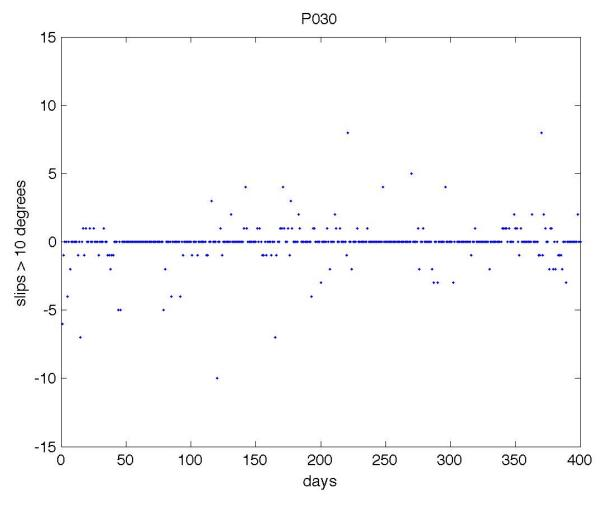
We have observed that for elevation angles  $< 10 {\hat A}^{\varrho}$  the mean difference between the number of slips for L2C and L2P phases is ~7.7 slips over a 400 day period. Tracking L2C increases the number of observations, but it also increases the number of slips for elevation angles  $< 10 {\hat A}^{\varrho}$ .
