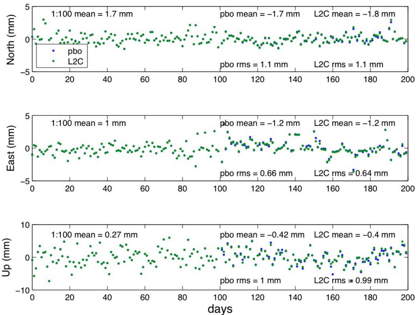
The mean differences between the position time series are  $< \sim 0.1$  mm in the horizontal and  $< \sim 0.2$  mm in the vertical components (shown below).
