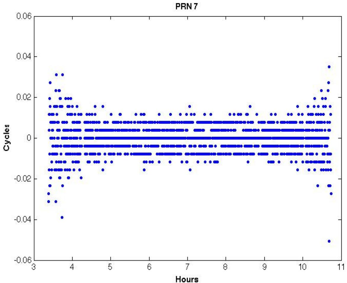
The difference between each band in the figure above is  $\sim 0.0039$  ( $1/256$ ) cycles. This banding demonstrates that the digitizing resolution of the NetRS receiver is  $1/256$  ( $1/2^8$ ) of a cycle - implying that the receiver is using an 8 bit A-D conversion. The analysis above was done using a translation of RT27-format data using extended resolution on the phase values beyond the usual 0.001 cycle resolution available in RINEX observation format.
