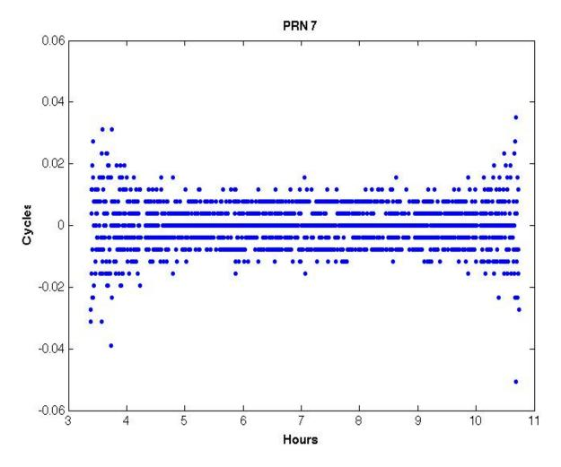
The difference between each band in the figure above is ~0.0039 (1/256) cycles. This banding demonstrates that the digitizing resolution of the NetRS receiver is 1/256 (1/2^8) of a cycle - implying that the receiver is using an 8 bit A-D conversion. The analysis above was done using a translation of RT27-format data using extended resolution on the phase values beyond the usual 0.001 cycle resolution available in RINEX observation format.
