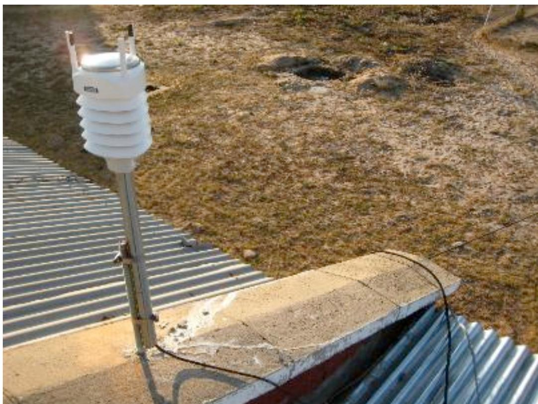
Example 1 - Vaisala hose clamped to  $\frac{5}{8}$  inch rod grouted into roof.
