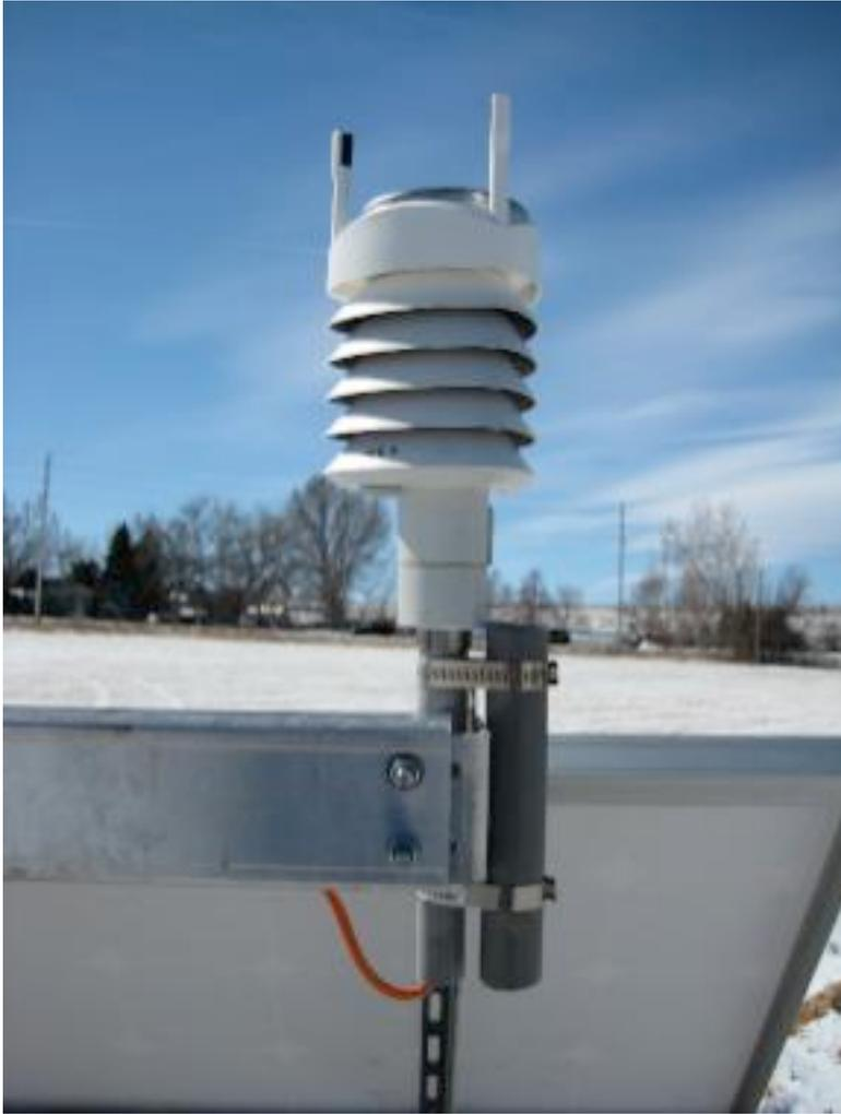
Example 3 - Vaisala mounting pipe is hoseclamped to an adjacent section of PVC, against a solar panel mount.
