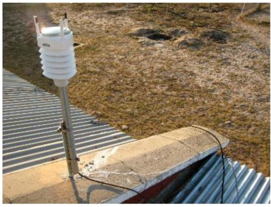
Example 1 - Vaisala hose clamped to 5/8 inch rod grouted into roof.
