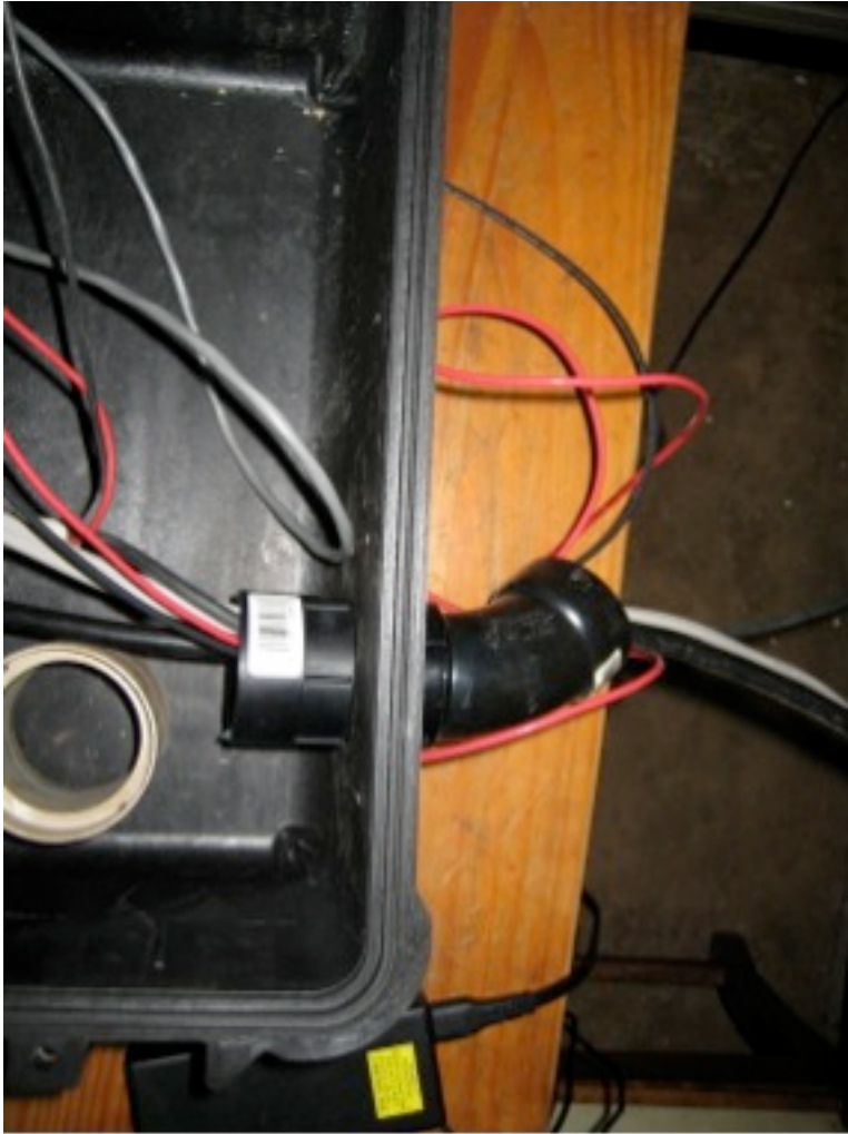
Plastic two" pass-through for cables routed from the GPS antenna, Vaisala weather station, solar panel, and battery
