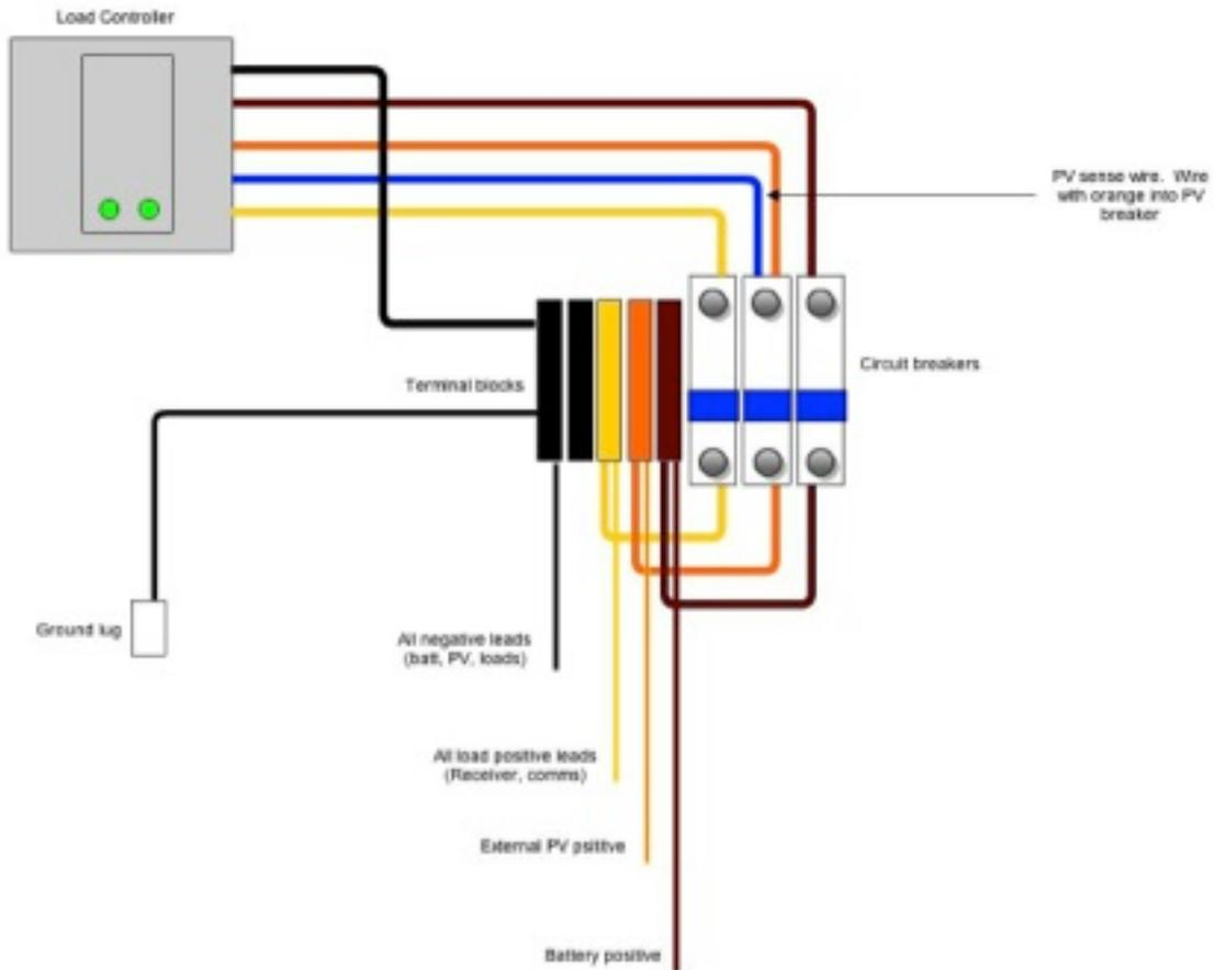
Backpanel wiring diagram
