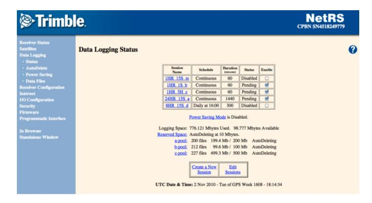
If you encounter receivers in this state, go to the "Receiver Configuration -> System Reset" and do a simple restart.
