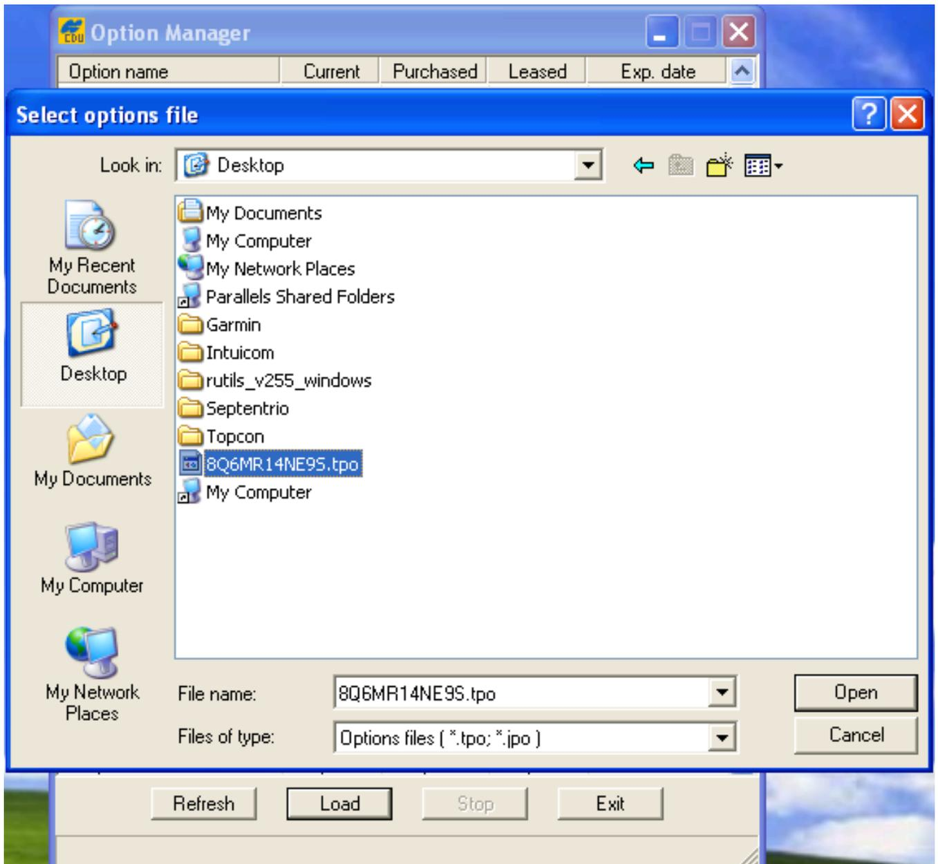
5. Click "Open" after selecting the proper file. If the load is successful you will quickly see the following screen, followed by a receiver reset and disconnection:
