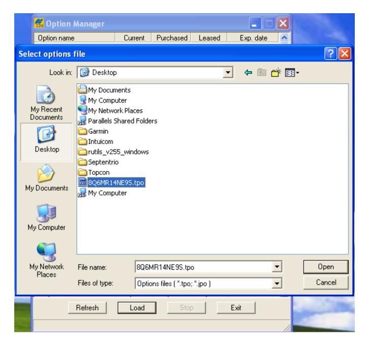
5. Click "Open" after selecting the proper file. If the load is successful you will quickly see the following screen, followed by a receiver reset and disconnection:
