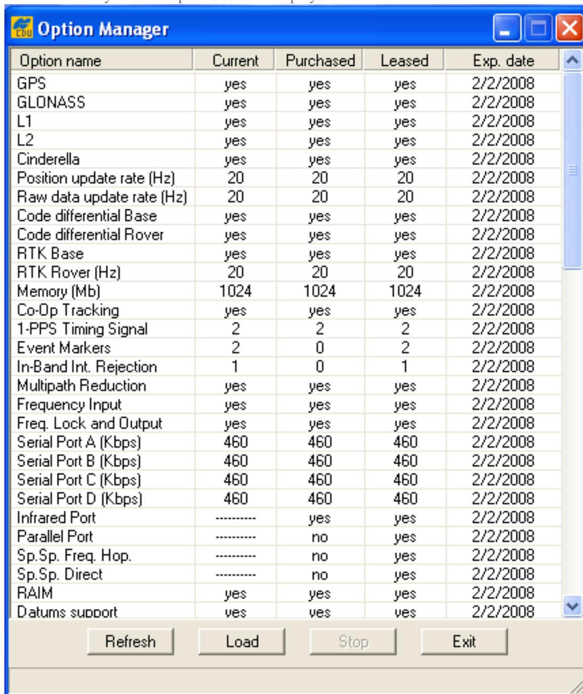
4. Select the new options file on your hard drive. Note that the file should be named according to the receiver ID shown on the window of the main PC-CDU screen:
