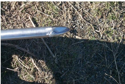
18. Place 4 tubes of epoxy in one of the slant leg holes and insert leg. Mate the slanted leg to the vertical leg and tack weld.
