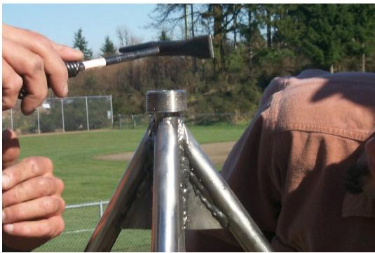
24. Weld the screw thread end of the of the SCIGN adaptor to the center leg.
