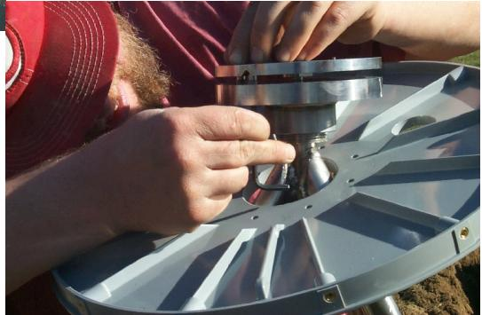
29. Thread the antenna bolt up through the top plate and finger tighten with a wrench. If using a Trimble legs using wire ties or hose clamps. [Note: Foam insulation used to isolate mount legs from soil.]
