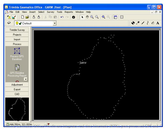
conventional survey data. Designed for ease of use, high productivity and quality control, the software imports, checks, and processes field data. The data is stored in Microsoft Access database format for easy customized access, reporting, and editing.
