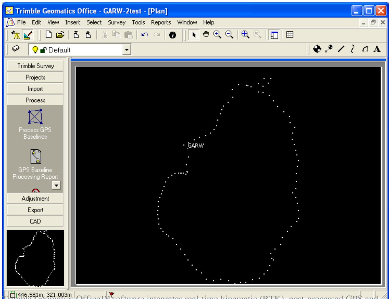
Trimble Geomatics Office™ software integrates real-time kinematic (RTK), post-processed GPS and conventional survey data. Designed for ease of use, high productivity and quality control, the software imports, checks, and processes field data. The data is stored in Microsoft Access database format for easy customized access, reporting, and editing.
