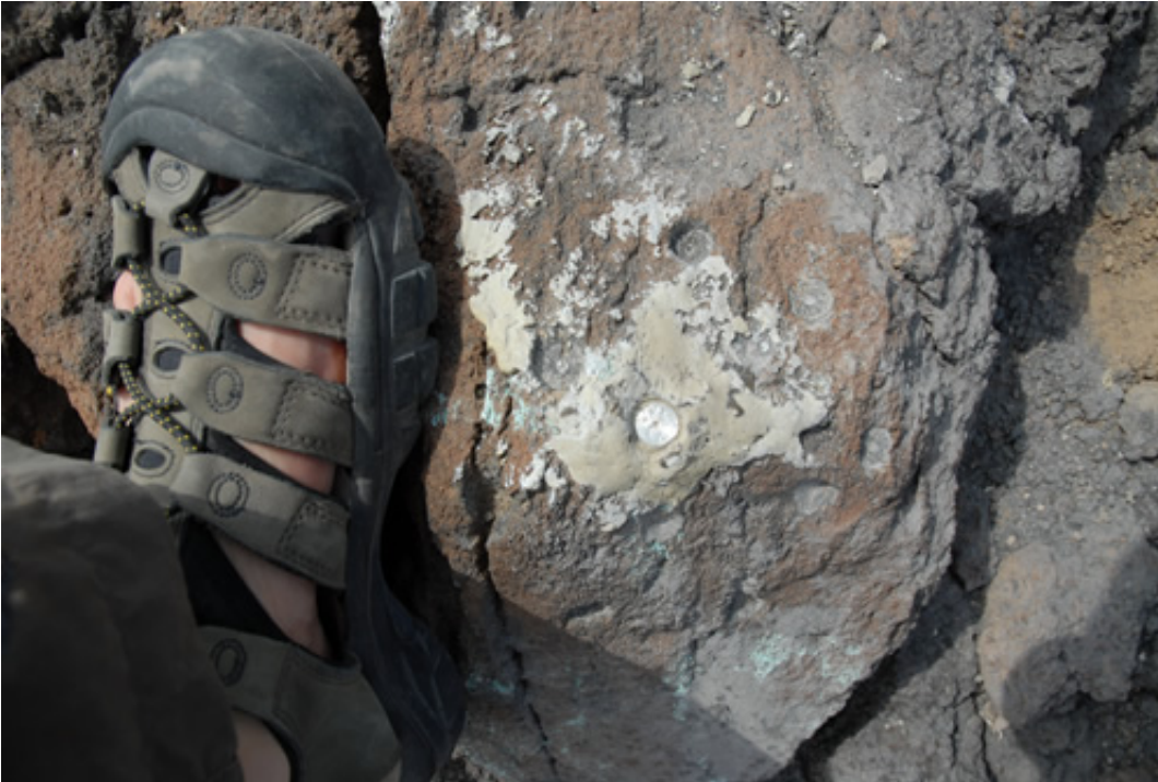
Danish geodetic marker near Kangerlussuaq, Greenland (left); simple stainless steel pin at site DOIW in Afar, Ethiopia (right).
