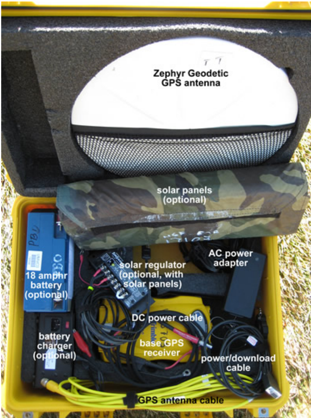
UNAVCO NSF EAR RTK base GPS unit: typical packing (left) and view of all components (right).
