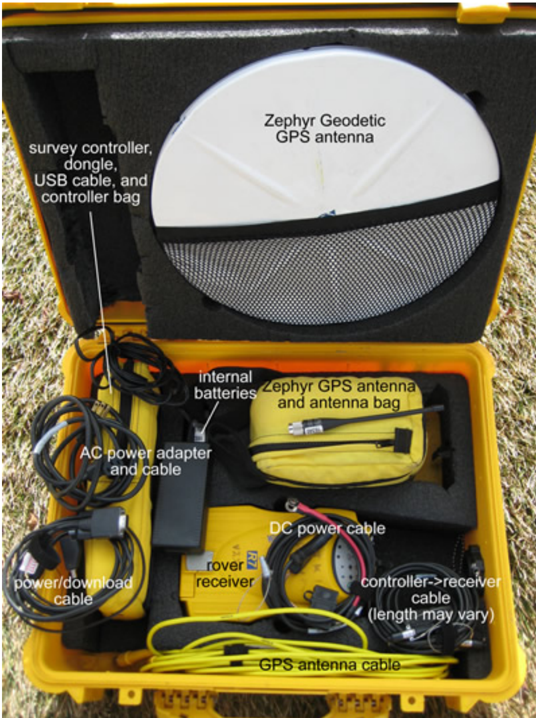
UNAVCO NSF EAR RTK rover GPS unit: typical packing (left) and view of all components (right).
