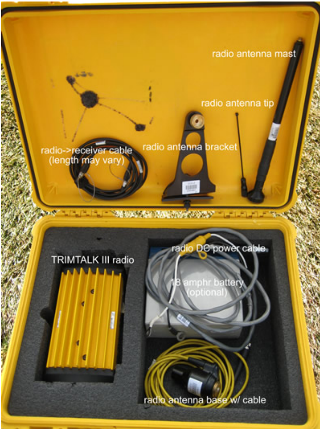
UNAVCO NSF EAR RTK base radio unit: typical packing (left) and view of all components (right).
