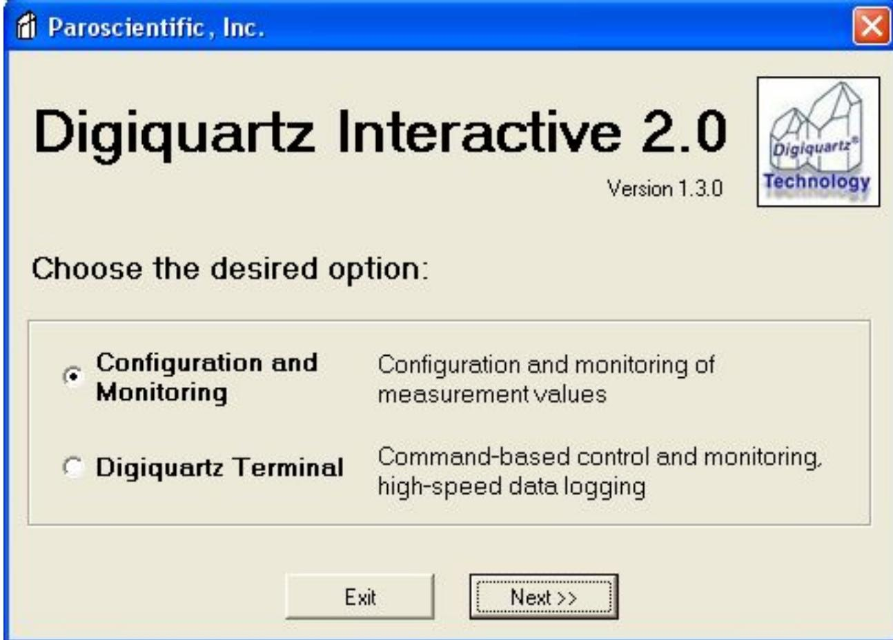
At this point you have two options. You can go into "Configuring and Monitoring" or "Digiquartz Terminal". The first option will take you into a more user-friendly, menu-driven configuration and plotting window. The "Digiquartz Terminal" will take you to a blank window where you can send commands such as \*0100P9 to the MET4. Both of these features of Digiquartz Interactive 2.0 are needed to configure the MET4.
