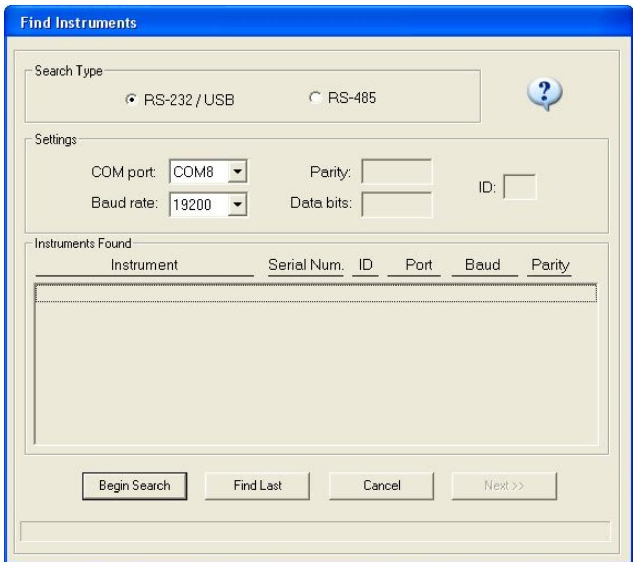
Select the mode in which you are connected to the MET4. In this case we are connected with a serial cable on COM8 with a baud rate of 19200. In the case you don't know the baud rate or COM port you can simply select "Begin Search"; Digiquartz then cycles through all combinations of COM ports and possible baud rates until it finds the MET4.
