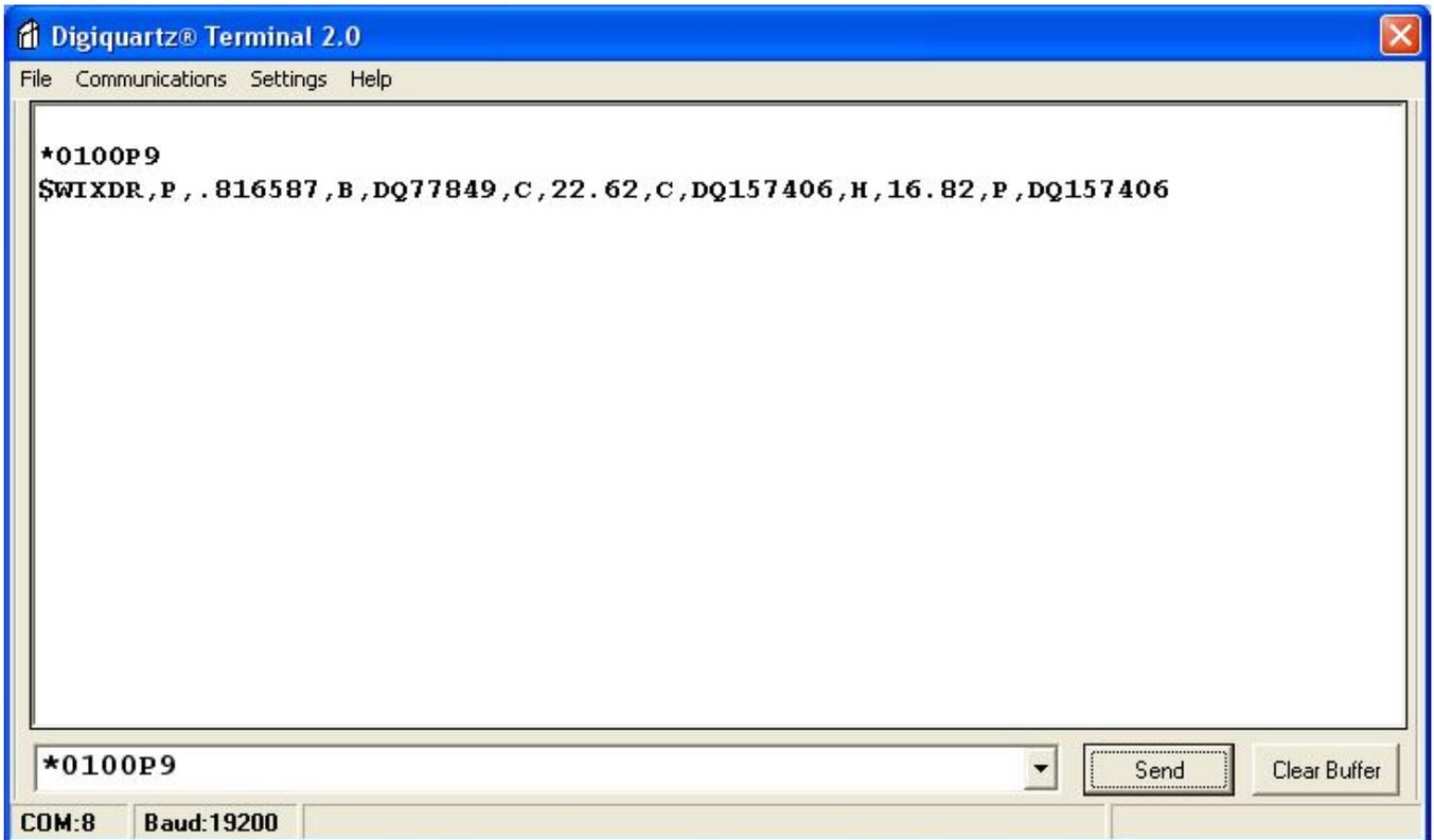
The P9 response is divided into a header and three measurement sections (pressure, temperature, and humidity). Each measurement consists of an identifier, a measurement value, a unit, and a transducer serial number separated by commas.
