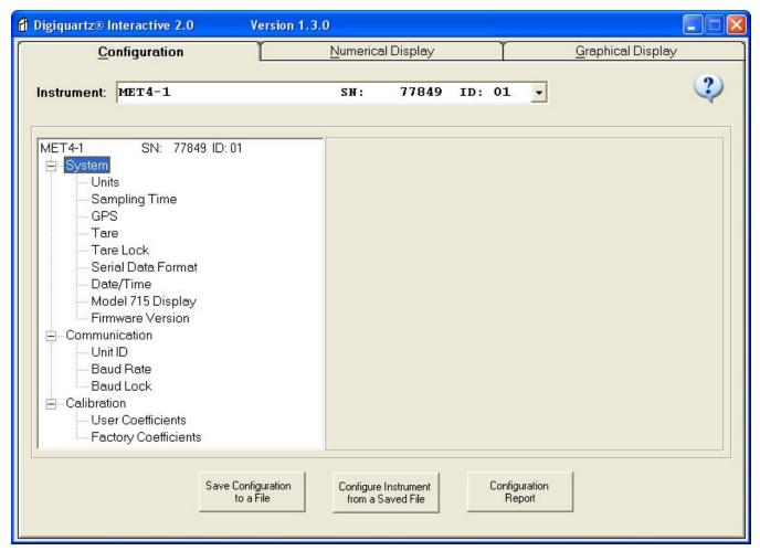
If the GPS receiver will be querying the MET4 for Temperature, Pressure and Humidity with \*0100P9 the MET4 will NOT respond unless the Pressure Units are set to "bar".
