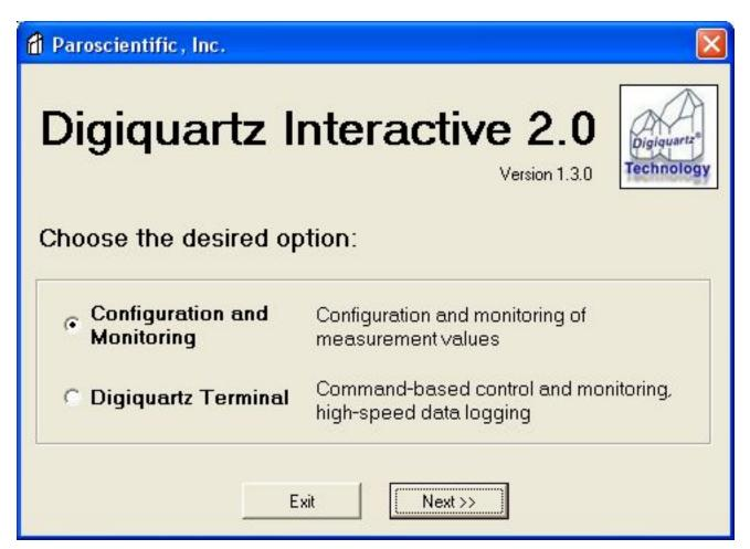
At this point you have two options. You can go into "Configuring and Monitoring" or "Digiquartz Terminal". The first option will take you into a more user-friendly, menu-driven configuration and plotting window. The "Digiquartz Terminal" will take you to a blank window where you can send commands such as \*0100P9 to the MET4. Both of these features of Digiquartz Interactive 2.0 are needed to configure the MET4.
