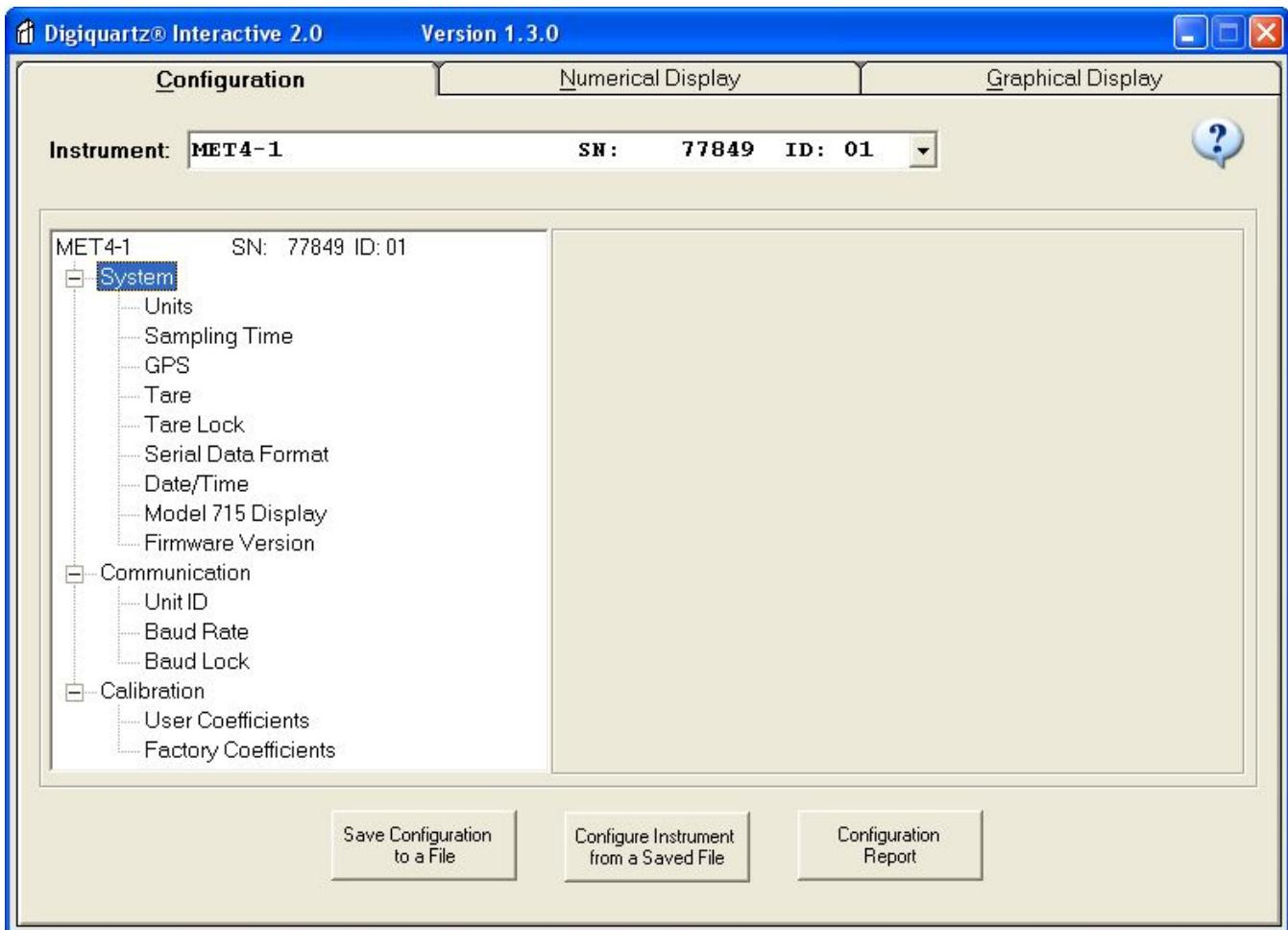
If the GPS receiver will be querying the MET4 for Temperature, Pressure and Humidity with \*0100P9 the MET4 will NOT respond unless the Pressure Units are set to "bar".
