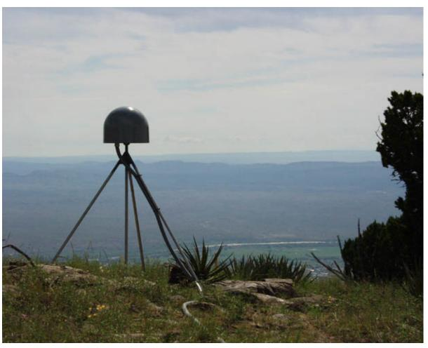
Configuration 3 - Standard atmospheric or atmospheric/geodetic site with a radio modem link
