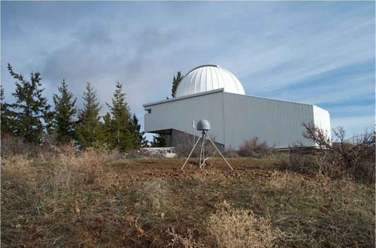
GPS station looking North. The UW observatory is in the background. MET sensor can be seen directly behind the GPS antenna.
