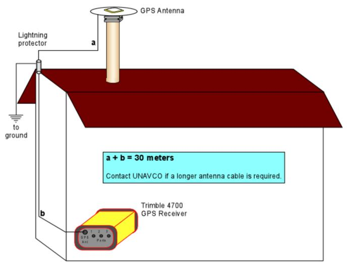
For cable runs longer than 30m custom cables must be used. Obtaining these cables is the responsibility of the participant. The total cable loss can not exceed 12dB.
