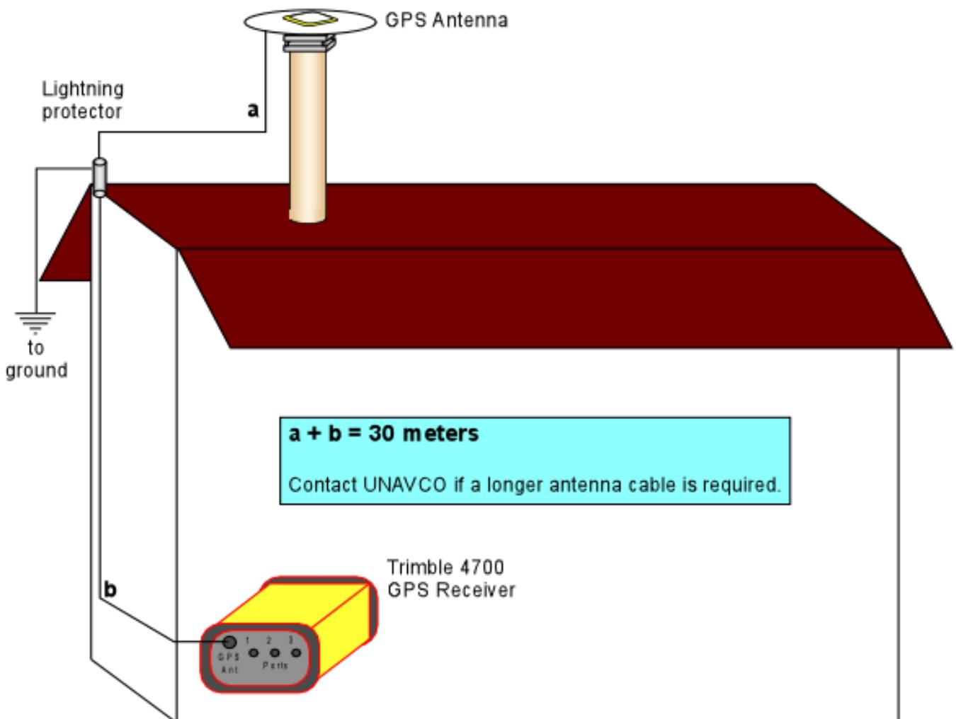
For cable runs longer than 30m custom cables must be used. Obtaining these cables is the responsibility of the participant. The total cable loss can not exceed 12dB.
