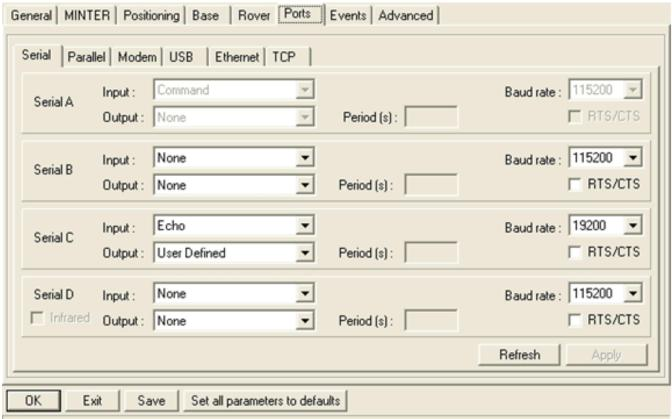
Figure 1: Since we connected the MET3 to serial port C on the back of the receiver we have set that serial port to communicate with the MET3 at the same baud rate we set the MET3 to be. We have also selected the Input to be Echo and the output to be User Defined. Make sure you DO NOT select RTS/CTS.
