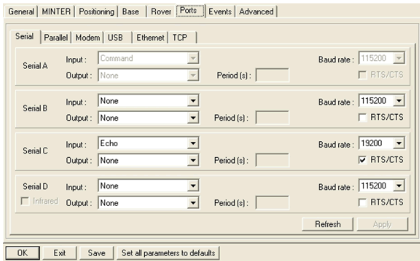
Figure 10: Since we connected the WXT520 to serial port C on the back of the receiver we have set that serial port to communicate with the WXT520 at the same baud rate we set the WXT520 to be. We have also selected the Input to be Echo and the output to be None. Make sure you DO select RTS/CTS.
