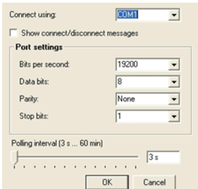
Figure 1: COM port settings for communicating with a WXT520 using the Vaisala Configuration Tool.
