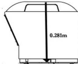
Vertical Offset from GPS antenna mount (bottom center of bolt) to ILRIS 0,0,0 is 0.281m
