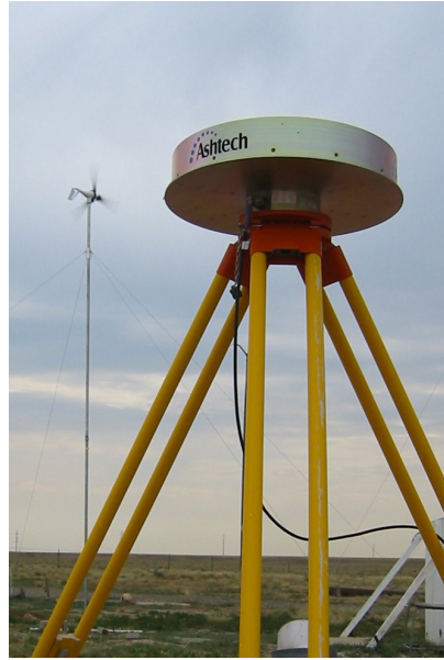
GPS Antenna w/ AIR 403
