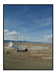
System: The Marshall Test site contains a power system which includes a battery bank, solar and wind charging systems. A permanant VSAT dish is located to test VSAT control boxes before they are sent out. Various receivers and radio modem systems are also tested at this location.
