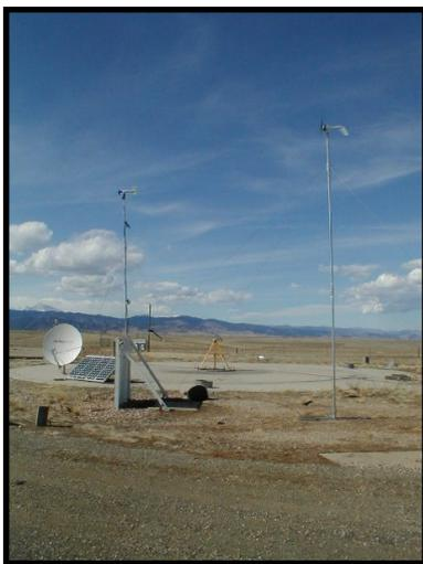
**System:** The Marshall Test site contains a power system which includes a battery bank, solar and wind charging systems. A permanent VSAT dish is located to test VSAT control boxes before they are sent out. Various receivers and radio modem systems are also tested at this location.
