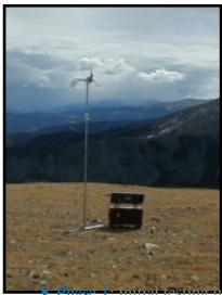
Phase 1: Initial testing in high wind environment. Establish base test parameters and identify any initial system issues. 4/02-6/02
