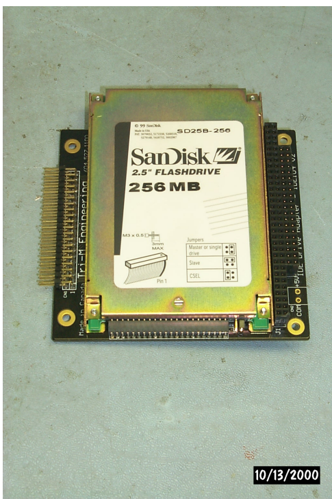
Hard drive fixed onto the hard drive adapter board. Hard drive adapter board provides power to the drive through the PC/104 plug. This adapter board also provides a standard IDE connector.
