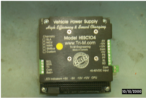
Top view of the UPS power supply controller, already bolted onto the battery bank board.
