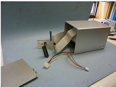
Showing how the back of the box comes off in order to connect the system to a floppy drive, a CD-rom, and connects the system to power.
