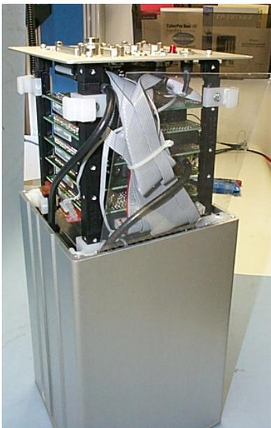
A piece of plastic film is used to prevent wires from getting tangled and torn while putting the frame casing into the box.
