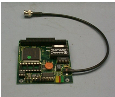
10 base 2 ethernet board.
