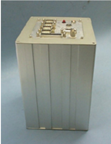
The entire PC/104 system in its casing.
