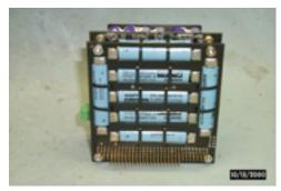
Nickel Cadmium batteries 7AA x 0.6A hr. with digital temperature sensor 3.78" x 3.5" x 0.592" (L x W x H) Weight: 7.78 oz / 220.45 grams Temperature range: -20 to +60 C
