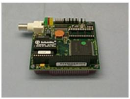
NE2000 Compatible PC/104 Ethernet Controller Uses National AT/LANTIC<sup>TM</sup> High Integration Controller
