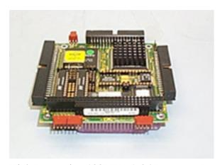
High Integration 133MHz 5x86 Processor Board PC/104 Sized Module
