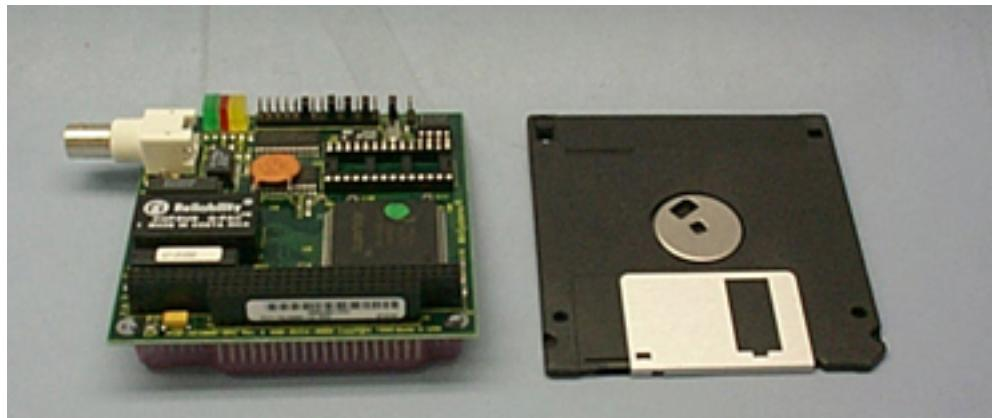
Ethernet board with BNC coax is shown next to a floppy disk for size comparison.
