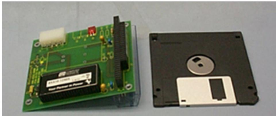
DC to DC Inverter board shown next to a floppy disk for size comparison.
