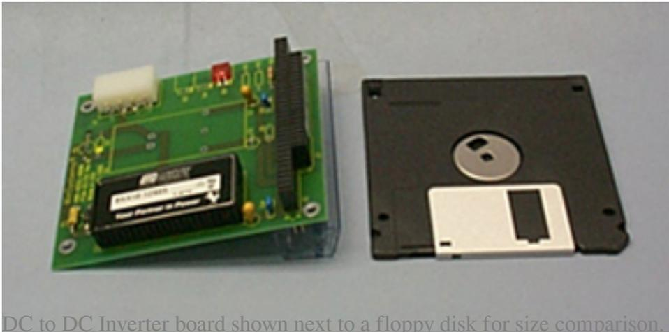
DC to DC Inverter board shown next to a floppy disk for size comparison.
