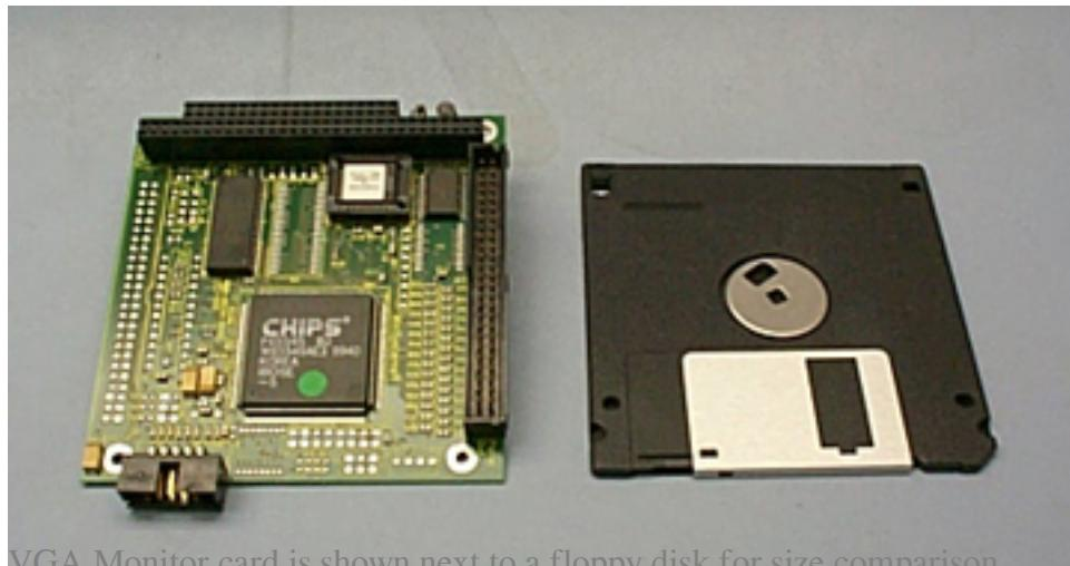
VGA Monitor card is shown next to a floppy disk for size comparison.
