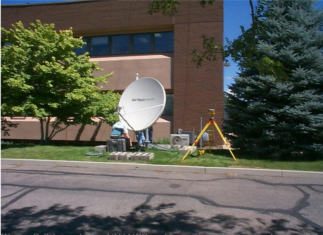
Warren Gallaher and other UNAVCO engineers using a spectrum analyzer to find the satellite signal.
