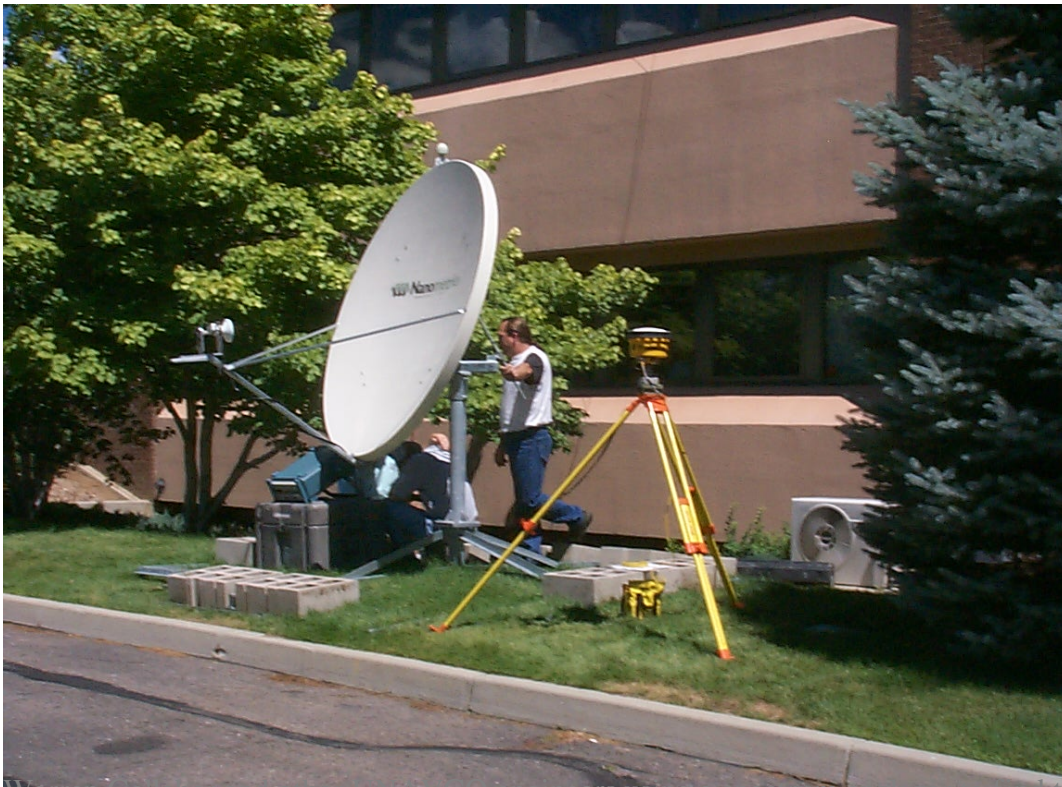
Warren Collins, UNAVCO engineer, adjusting the tripod to receive the satellite signal.
