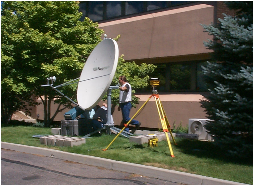
Warren Collins, UNAVCO, Boulder facility of Edouard engineers using a precision antenna to receive the satellite signal.
