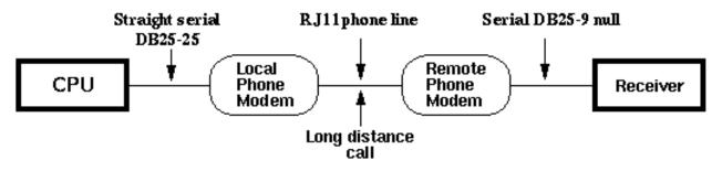
**NOTE:** Download rates will vary depending upon site location, local interference, phone line quality, and cellular service. The remote modem (at the GPS receiver) is configured the same as the local modem (at the download computer), but with remote modem file transfer protocol and modem set to pick up after one ring.
