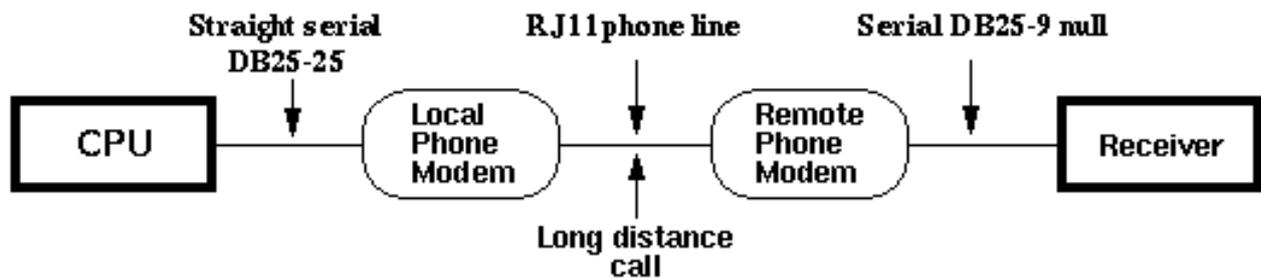
**NOTE:** Download rates will vary depending upon site location, local interference, phone line quality, and cellular service. The remote modem (at the GPS receiver) is configured the same as the local modem (at the download computer), but with remote modem file transfer protocol and modem set to pick up after one ring.
