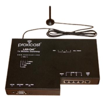
Proxicast CDMA modems are being utilized for data downloading of Trimble NetRS GPS receivers at permanent GPS stations in the Western United States.
