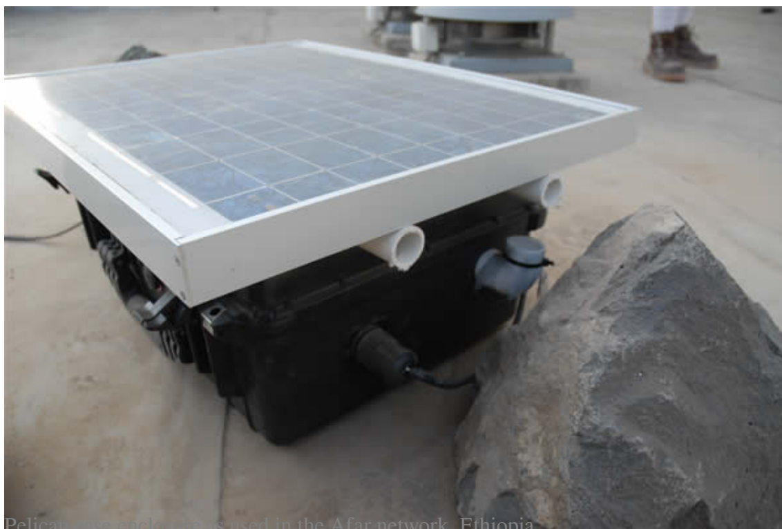
Pelican case enclosure is used in the Afar network, Ethiopia.
