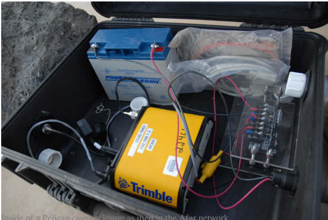
Inside of a Pelican case enclosure as used in the Afar network.
