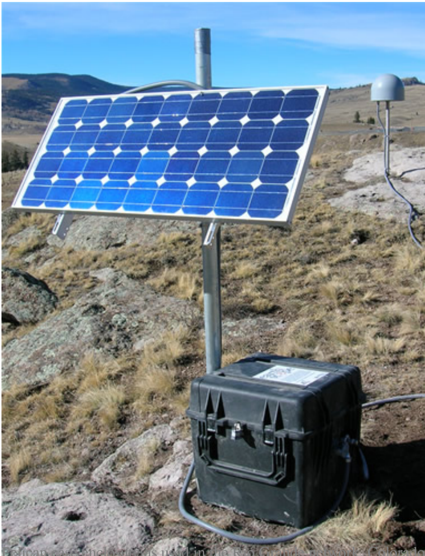
Pelican case and solar panel as used in the Red Clouds, Colorado and New Mexico.
