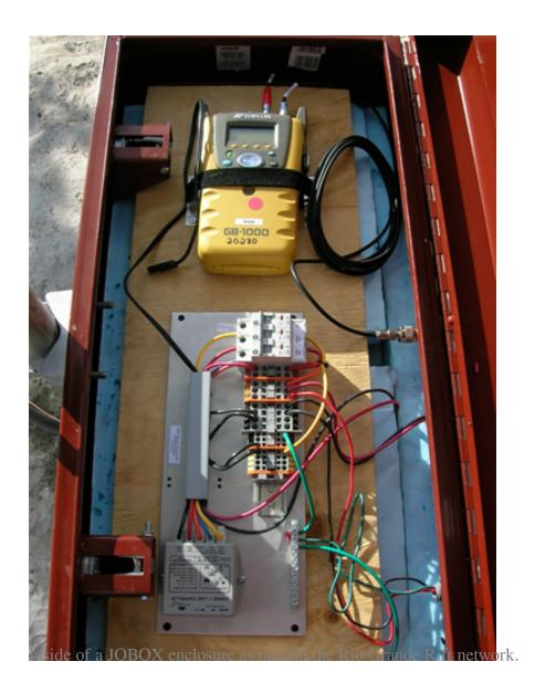
JOBOX chests, made by <u>Delta Consolidated Industries</u>, <u>Inc.</u>, are durable, weatherproof metal enclosures that UNAVCO has used in several long-term installations, including the EarthScope-sponsored Rio Grande Rift network. Chests are secured with key locks. The major drawback of the JOBOX is weight; boxes are heavy and cumbersome, thus not ideal for shipping and for transporting by foot over long distances. Cost of the box shown here is approximately \$300-400 (as of February 2009).
