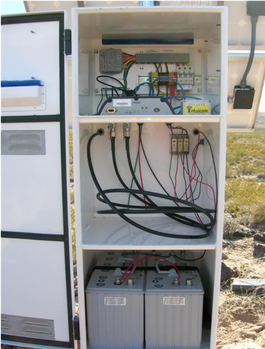
Inside of a SunWize enclosure as used in the Plate Boundary Observatory and in the BARGEN network.
