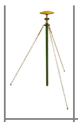
benchmark's central point and the mast is secured and leveled by adjusting the tension of the chains. Segments allow for multiple height options. A level is included in the Tech 2000 kit; a compass is needed for installation. The Tech 2000 is lightweight and highly portable, but requires a hand drill for setting anchor points for the first site visit. Used for non-permanent long-term and campaign sites.
