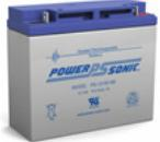
**18 amp hr battery (12 volts)** - Will power the receiver and GPS antenna for approximately 2 days in optimal conditions. Battery life decreases significantly in cold weather. Do not allow conductive material (e.g. a piece of metal) to contact both terminals at the same time as this will short the battery.
