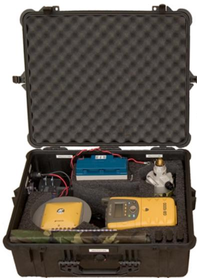
NSF's EarthScope Science panel. The systems have been designed for stand-alone temporary or semi-permanent deployment that will be used for densifying areas not sufficiently covered by continuous GPS and for responding to volcanic and tectonic crises. Six of the 100 systems are equipped with real-time kinematic (RTK) capability for such uses as rapid fault mapping and GIS-based geologic mapping. For [EarthScope campaigns](#) only. Antenna mounts must be requested separately.
