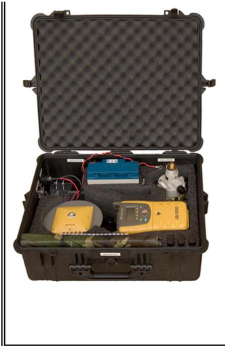
NSF's EarthScope Science panel. The systems have been designed for stand-alone temporary or semi-permanent deployment that will be used for densifying areas not sufficiently covered by continuous GPS and for responding to volcanic and tectonic crises. Six of the 100 systems are equipped with real-time kinematic (RTK) capability for such uses as rapid fault mapping and GIS-based geologic mapping. For [EarthScope campaigns](#) only. Antenna mounts must be requested separately.
