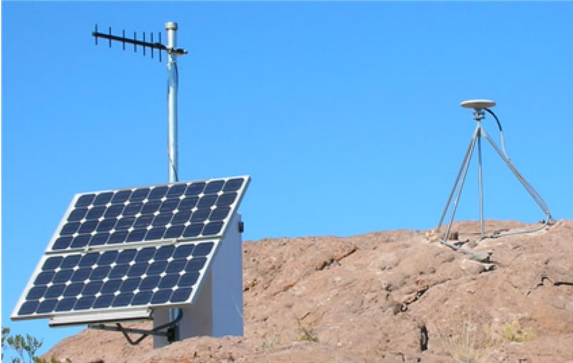
A Yagi antenna is used to transfer data via CDMA modem from site CDVV near Socorro, New Mexico to New Mexico Tech.
