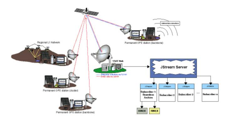
**Figure 1** VSAT network consisting of a Ku- band central hub and processing facility in Boulder. At the remote site, the Jstream java application would be used to convert the stream to BINEX before transmitting the data to a central hub. At the hub, Jstream would be run again to allow for distribution to
