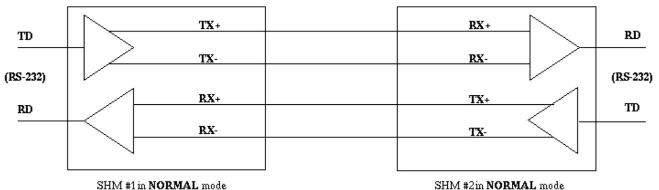
Figure 2: SHM-B Modem Test Configuration (Loopback Test)
